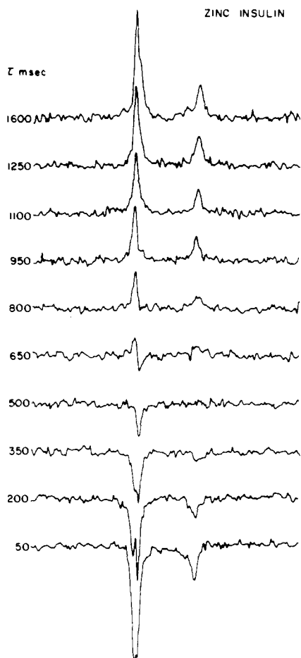
Figure 4. Proton-decoupled ^{13}\text{C} NMR partially relaxed Fourier transform spectra of carbamylated zinc insulin. See also caption of Figure 2. The number of transients per spectrum was 2000. The repetition time of the 180^\circ - \tau - 90^\circ pulse sequence was 4.4 sec. Delay times, \tau , between pulses are given in the figure.
